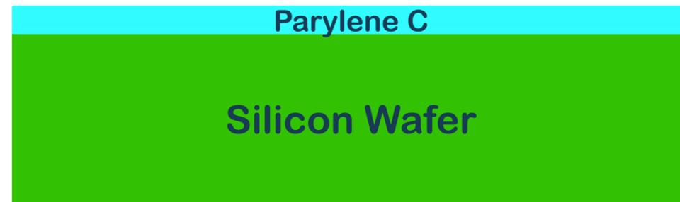
Deposition of 7 μm Parylene C layer on a 4" silicon wafer by means of a CVD process performed at room temperature
